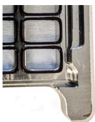
Figure 6 Correct positioning of gasket slide in chamber base
