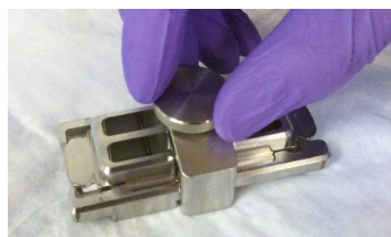
Figure 15 Loosening of the thumbscrew
