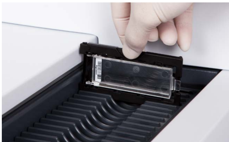
Figure 23 Inserting slide holder into cassette
