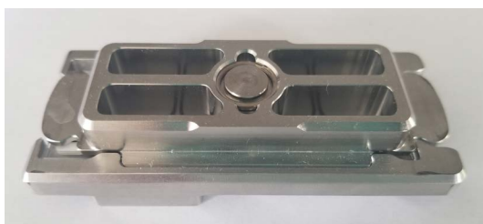
Figure 9 Chamber cover setting on chamber base in correct orientation
